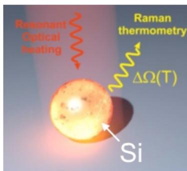
Fig. 1. Schematic illustration of strong optical heating and Raman thermometry of silicon nanoparticle.
