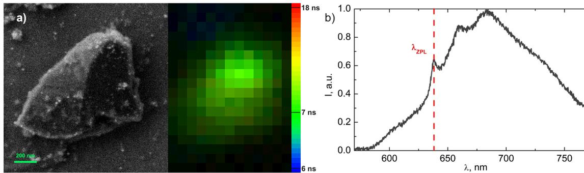
Fig. 1: a) Studied nanodiamond containing NV-center: left - the SEM image, right - the map of lifetime measurement; b) The photoluminescence spectrum
