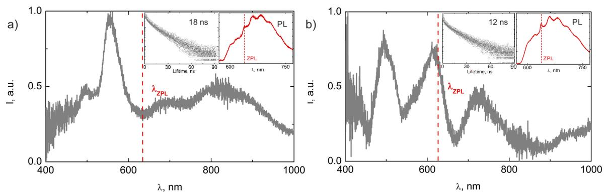
Fig. 2: The dark-field scattering spectra of nanodiamonds a) off-resonance case with the measured lifetime of 18 ns and b) resonance case with the measured lifetime of 12 ns. Insets: left - lifetime decay and right - photoluminescence for the off-resonance and resonance cases
